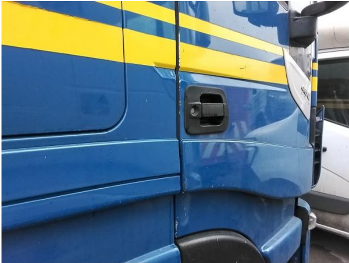
10: Door osf Scratched Over 25mm Thru Paint
