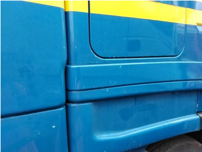
9: Qtr Panel osr Chipped Multiple Chips
