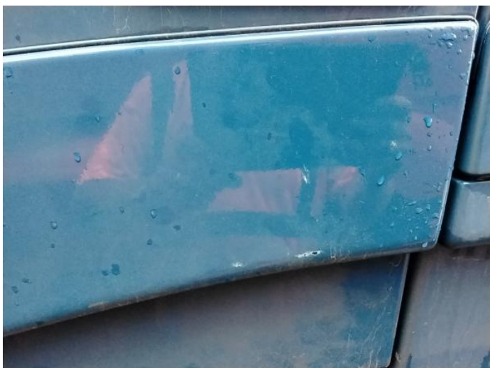
5: Door nsf Scratched Over 25mm Thru Paint
