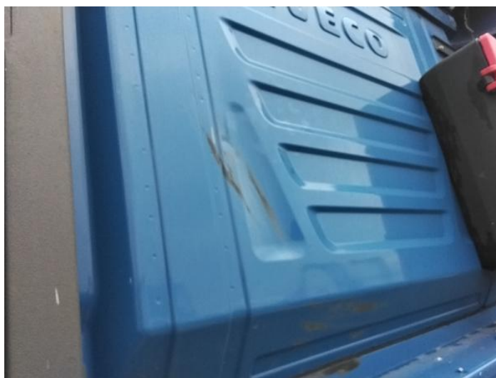
8: Panel Rear Dented Over 30mm
