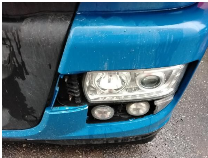
2: Bumper Front Moulding Missing Replace
