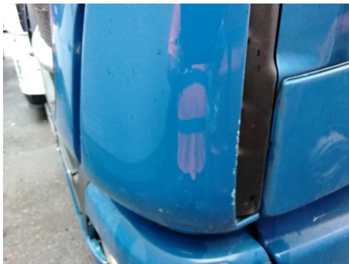
4: Panel Front Scratched Over 25mm Thru Paint
