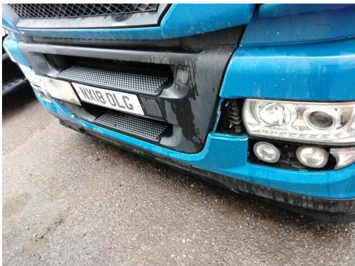
3: Bumper Front Chipped Multiple Chips
