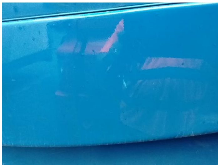
6: Door nsf Scratched Over 25mm Thru Paint
