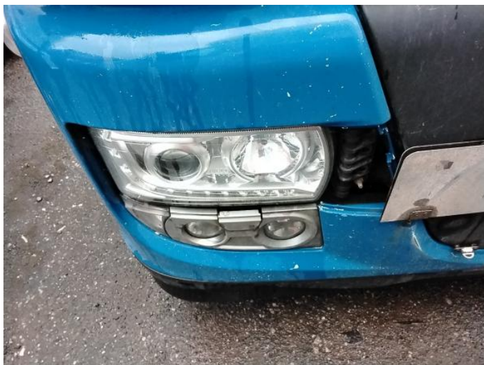
1: Bumper Front Moulding Missing Replace
