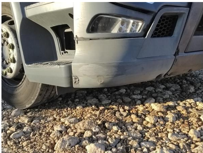
1: Bumper Front Moulding Scuffed (Unpainted) UpTo 100mm
