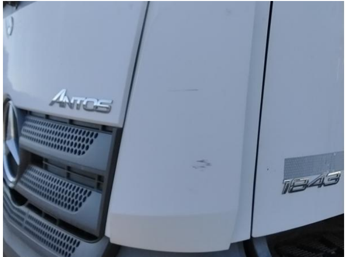
10: Wing nsf Scratched UpTo 25mm Not Thru Paint
