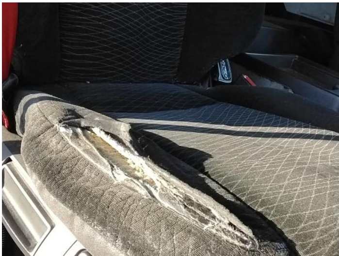
15: Seat Base Cover osf Torn Over 3mm
