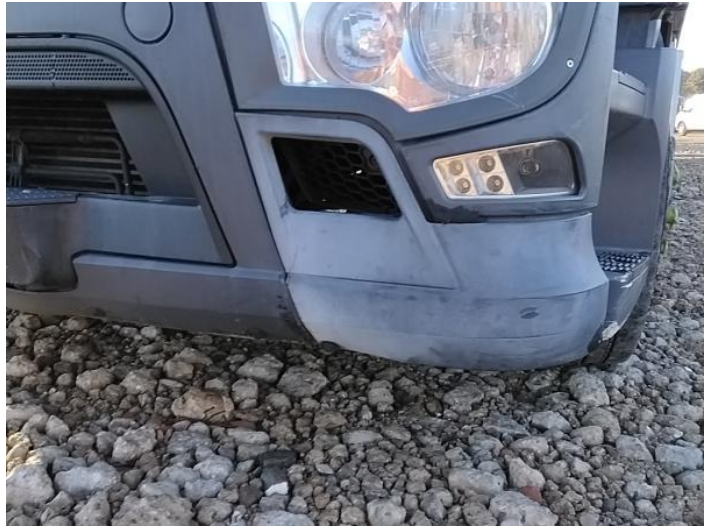
4: Bumper Front Moulding Scuffed (Unpainted) UpTo 100mm
