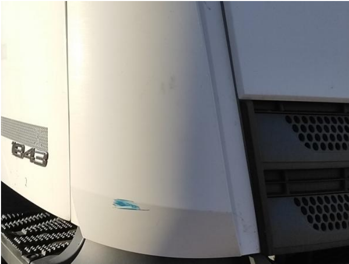
3: Wing osf Scratched UpTo 25mm Not Thru Paint
